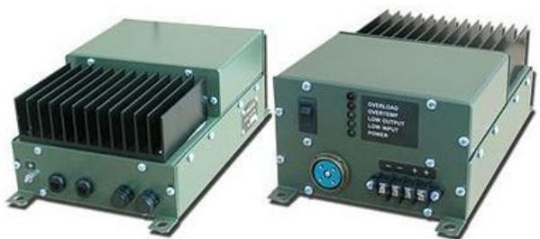
► The DC-DC (12V to 24V / 30A) converter is intended for use with military mobile radio stations and communication equipment with a supply voltage of 24 ... 30 VDC in cases where the vehicle's onboard voltage is 12...14 VDC.
