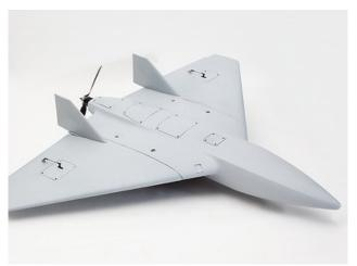
> In-house designed and manufactured UAV - Electro Raven. Electro Raven is easy to use, fast to assemble composite airframe electro drive UAV with various hatches for ease of access of internal compartments.
